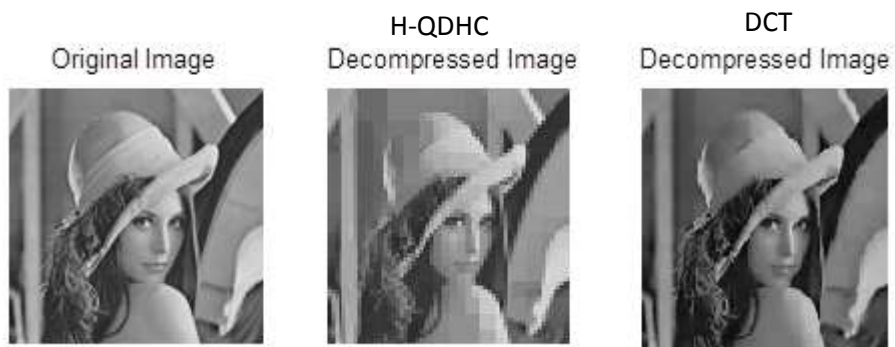
Figure.3.2 Comparison of visual image quality of reconstructed image for QDHC and DCT respectively
